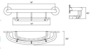
Easy to mount flange! Welded, 3" round, 5 hole flange with concealed cover.
