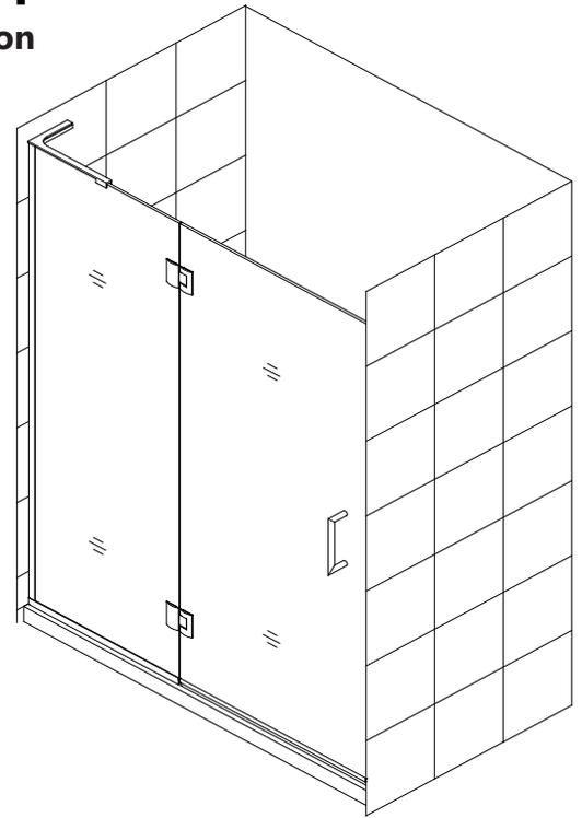
**1.** Trim the **0.5mm PVC glass spacer (#34)** into several 2" pieces. Insert three to four 2" pieces of the **0.5mm adjustment spacers (#34)** into the **U-channel 2 (#29) (bottom profile)**. These are used as setting blocks to protect the bottom of the glass.
