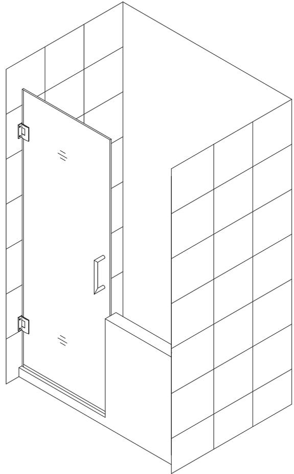
**NOTE:** The Unidoor hinge is designed to over close 8°. The following procedure is recommended to ensure proper alignment of the panel glass and door.
