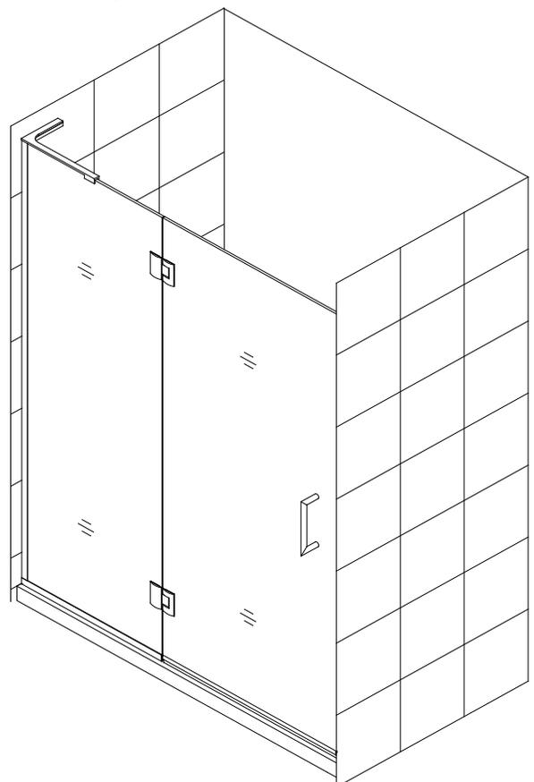
**14.** With the door open apply waterproof silicone along the connection of both U-Channels to the wall and threshold on the inside of shower.
