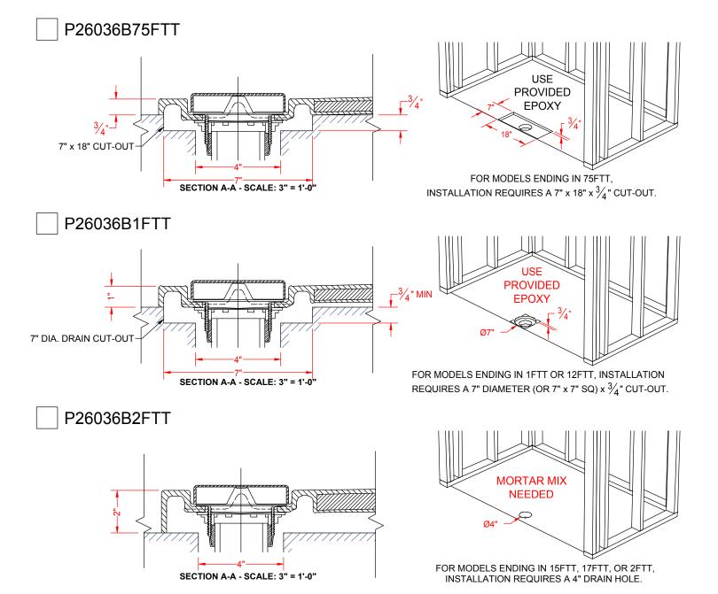
ALL SHOWN AS INSTALLED WITH SOLID BRASS, NO-CAULK DRAIN FITTING (INCLUDED, INSTALLED BY OTHERS)
