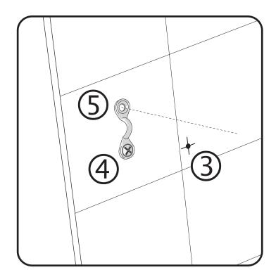
4. Put a small dab of 100% silicone over all holes, and insert the male snaps and the eye strap screws. Wipe away any excess silicone with paper towel or rag.
