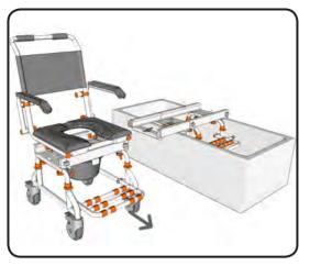
Ensure the primary brake securely locks your Tubbuddy in position on the wheeled base before disconnecting the bridge.
