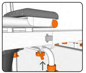
To transfer your Tubbuddy back to the wheeled base lift and hold the primary brake lever to release the chair. The primary brakes are located on each side of the wheeled and bath base tracks at the front.
