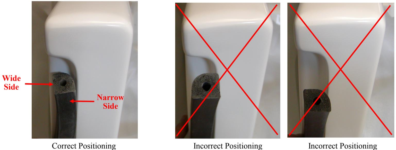
5. Beginning at one end of the seal, carefully place the seal into seal area of door taking care to make good contact between the door and seal. Be sure that the wide flat portion of seal is positioned as shown
