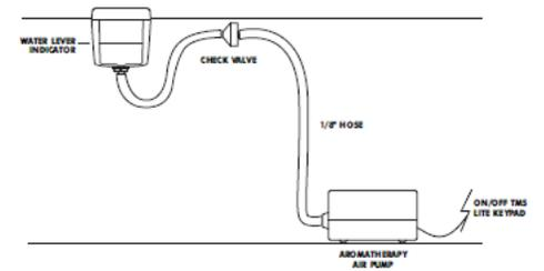
The system works using an air pump which leads the air towards the receptacle filled with water added with some essential oil drops.
