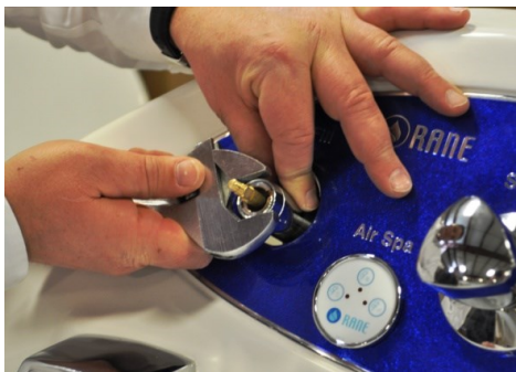
Step 5: Using a crescent wrench, remove part C (fig. 1).
