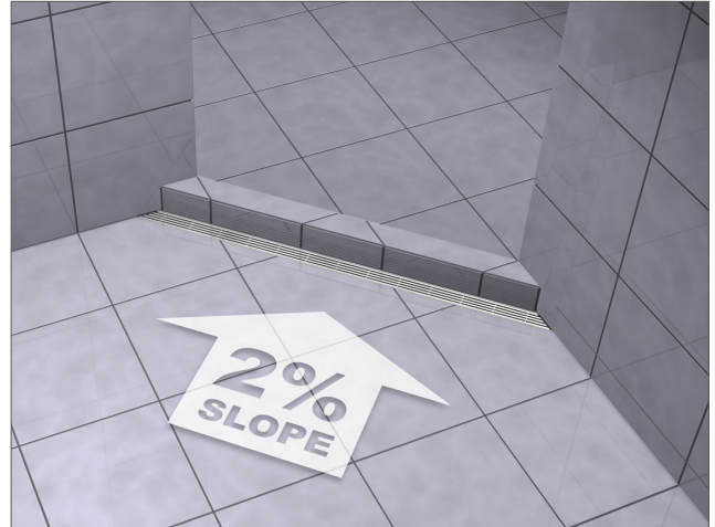
ProLine Drain at the shower entry right behind the curb.
