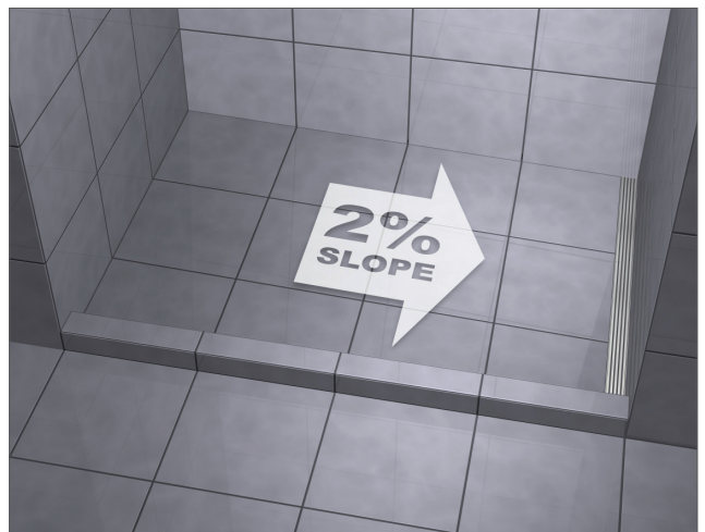
ProLine Drain at the side wall. Usually done when replacing a standard tub, because there is no need to move waste plumbing.
