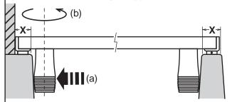
**BUMPER INSTALL.** If required, install the extra bumpers directly to the wood. Carefully drill a pilot hole for the (supplied) #6 pan head wood screws. Ensure the bumpers are aligned with factory-installed bumpers as shown in Bottom View.
