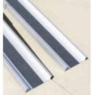
The TELESCOPIC CHANNEL RAMP is constructed of lightweight anodized aluminum with a black non-skid surface for traction. Useful for wheelchairs and some scooters, they have a wide 7½" usable track. Each channel extends to nearly double its length for fast and easy set up.
