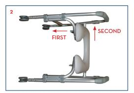
3. To install the backrest, insert backrest into backrest receptacles by depressing the brass pins on both sides into the commodes back frame. The brass push pins will snap into place when secure. Check by pulling back to insure the back is secure and locked into place
